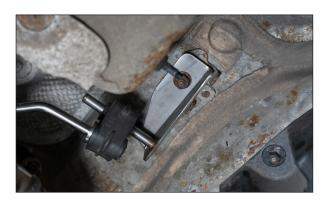
Replace both hangers with the ones supplied by Scorpion. Re-use the BMW rubbers or replace with new if deteriorated.
